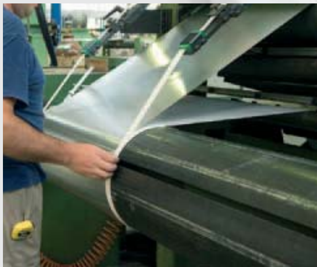
LV winding system
